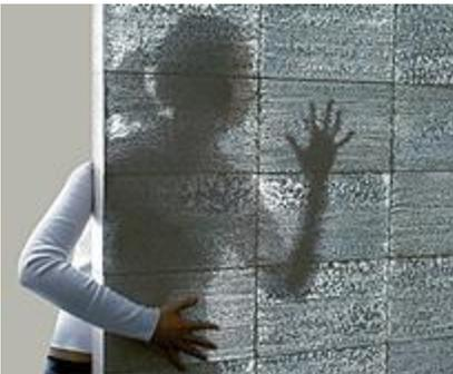
The glass fibers lead light by points between the two sides of the blocks. Because of their parallel position, the light-information on the brighter side of such a wall appears unchanged on the darker side. The most interesting form of this phenomenon is probably the sharp display of shadows on the opposing side of the wall. Moreover, the color of the light also remains the same.
