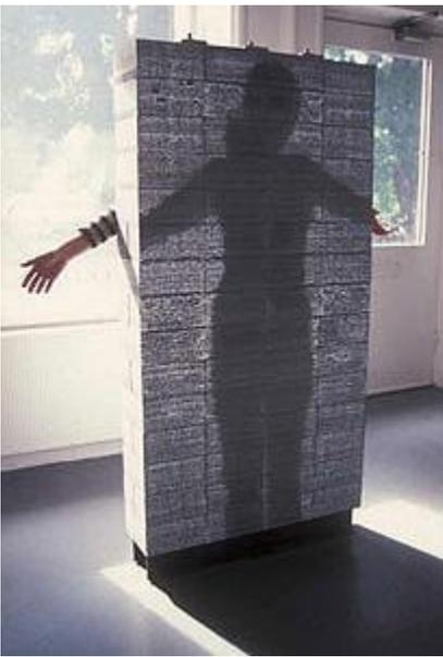
Litracon™ is a combination of optical fibers and fine concrete. It can be produced as prefabricated building blocks and panels. Due to the small size of the fibers, they blend into concrete becoming a component of the material like small pieces of aggregate. In this manner, the result is not only two materials - glass in concrete - mixed, but a third, new material, which is homogeneous in its inner structure and on its main surfaces as well.
